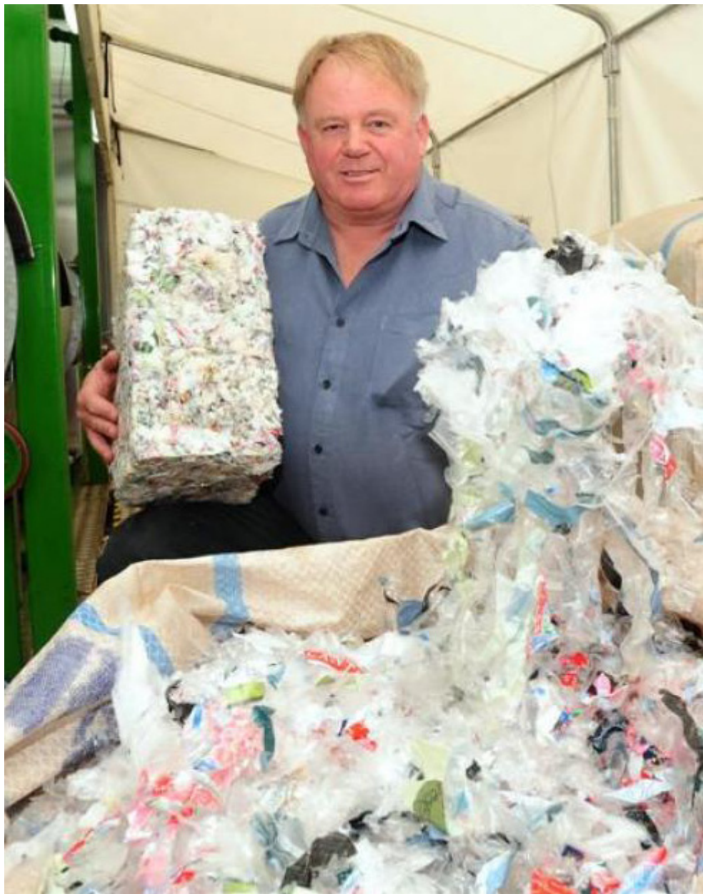
Peter Lewis' Byblock fusion invention turns bags of plastic waste into the equivalent of the standard concrete building block.
